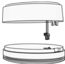
Remove the back cover from the Ei Electronics detector. The GSM communicator will be used as back cover. Press the green cabled connector to the pins of the Ei Electronics detector. Next to the pins the text 1 2 is written. Be sure that the (in most situations) grey connector in the Ei Electronics detector was removed.
