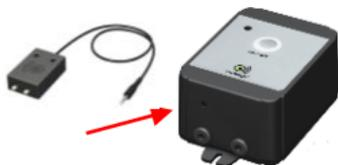
In case the sensor should detect the absence of water, the input type needs to be changed to NC (please refer to paragraph 5.4).
