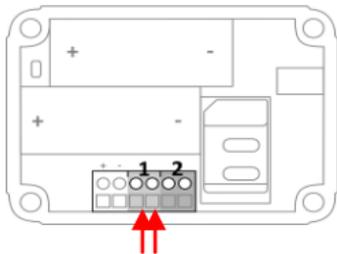
When using a second input, connect this to input 2.
