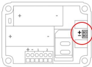
To switch devices, a relay can be placed behind the output with an input voltage of 12VDC. The required switching voltage of the relay depends on the device connected. NOTE: The output does not work if the CML2255 is battery-operated.
