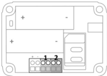
A second sensor can be connected to input 2.
