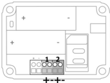
A second sensor can be connected to input 2.
