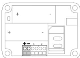
Using an external power supply the GSM module is always connected to the network. When there is a power failure, the batteries take over and power failure alarm messages are sent. The module continues operating albeit in the 'low power' mode. This means the GSM module switches off and only establishes network connection when it needs to send an alarm notification, test message or low battery alert.
