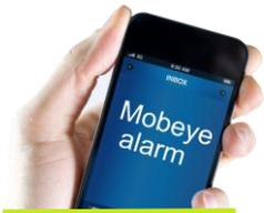
The Mobeye CM-Guard alerts with a telephone call, SMS and / or e-mail via the integrated GSM module. 'Confirmation' by the receiver will ensure that other contacts will not receive a call.
