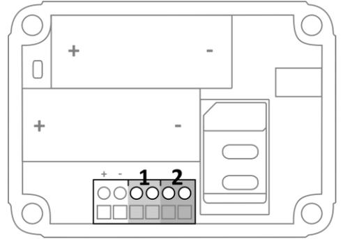
When using a second input, connect this to input 2.
