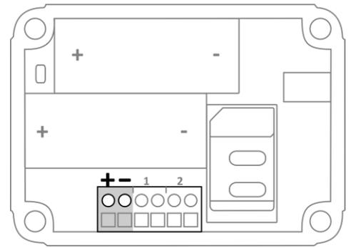
Connect the external power adapter (or any other regulated 12VDC power supply) to the power input of the connector (press on the green pins for connecting the wires):
