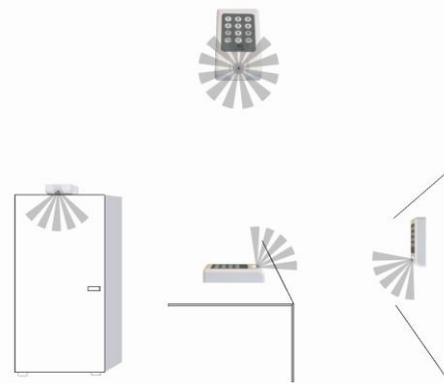
In order to check the reach of the sensor, a sensor test can be executed.
