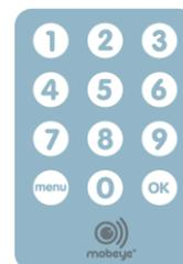
In case of false entries, the light turns red and a short beep will sound. The menu can be left from any position, by twice pressing “OK”.
